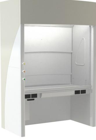
Flush Sill Airfoil With Containment Trough - Low-profile hinged Type 316 powder coated stainless steel airfoil is flush with work surface to provide ergonomic and unobstructed access to the interior. These include a built-in containment trough as an additional level of user protection from spills. Power cords can be run through the sill to the electrical outlets on the hood posts.
